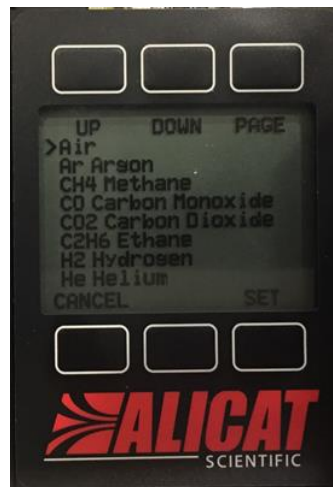
Alicat™ Mass Flow Controller Gas Select Display
