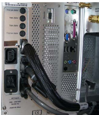
Figure 88 Disconnect the instrument power cable.
