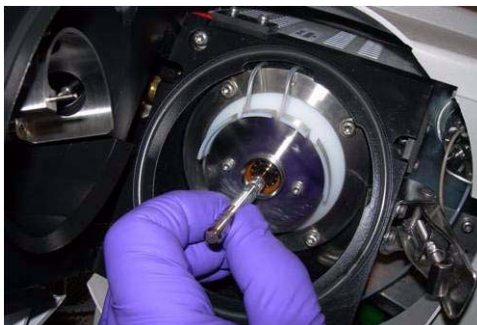
Figure 44 Pulling the capillary out of the desolvation assembly
