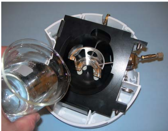
Figure 2 Filling the spray chamber
