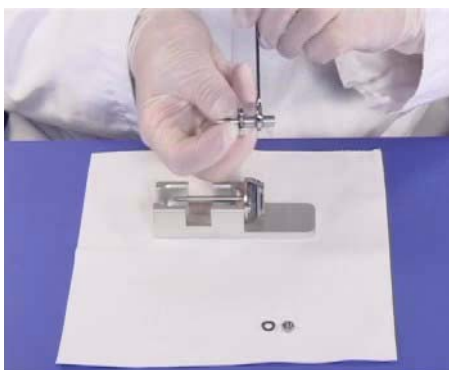
Figure 21 Tightening the union screw to compress the ferrule
