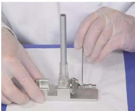
Figure 29 Installing the nebulizer in the adjustment fixture
