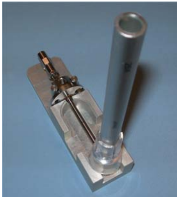
Figure 36 Electro spray nebulizer needle in needle holder
