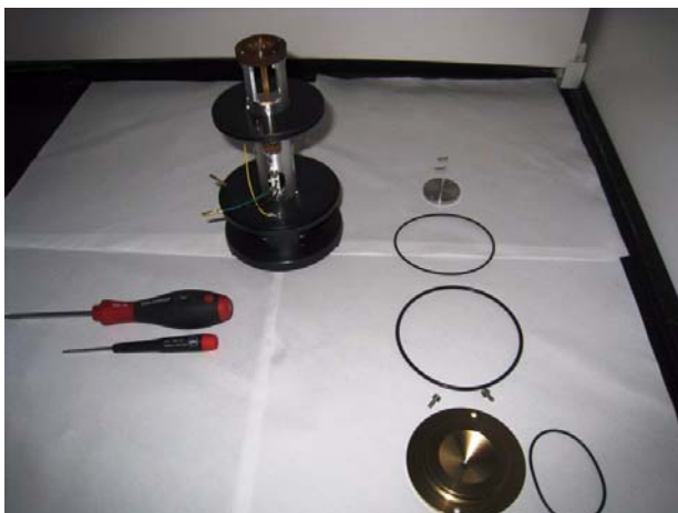
Figure 61 Skimmer and ion focus removed for cleaning
