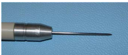
Figure 33 APCI corona needle after cleaning.
