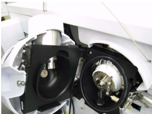
Figure 24 Opened spray chamber
