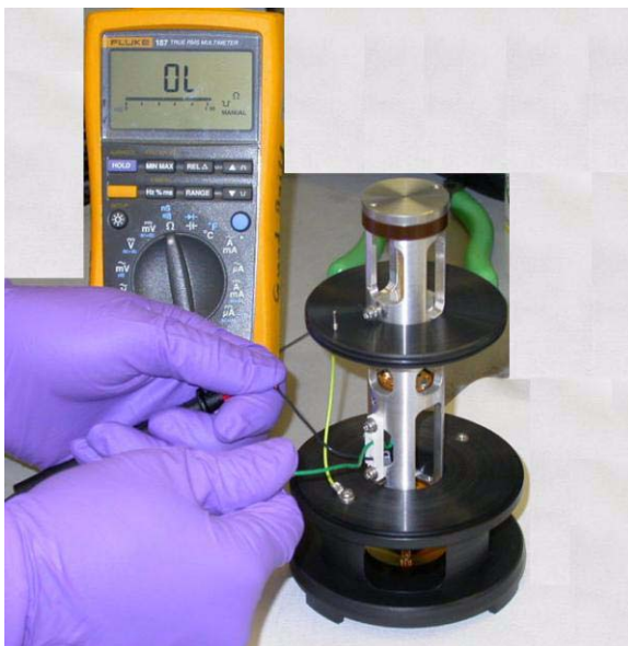
Figure 62 Testing for continuity.
