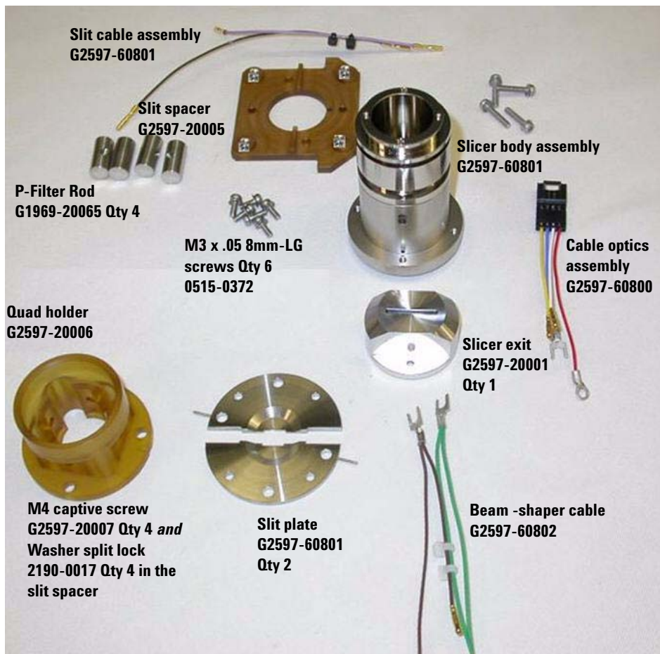
Figure 83 Slicer assembly part number identification.
