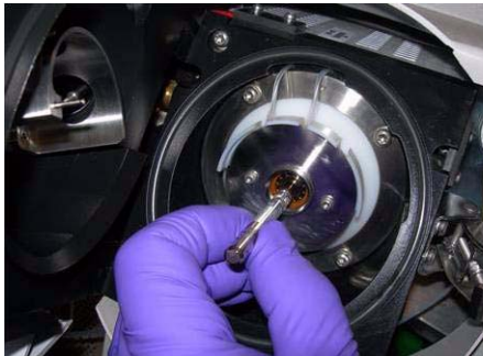
Figure 45 Reinstalling the capillary
