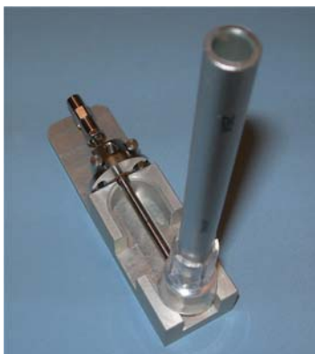
Figure 6 Electrospray nebulizer needle in needle holder
