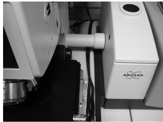
Figure 55: a) HYPERION 3000 connected to Spectrometer b) IMAC connected to HYPERION 3000
