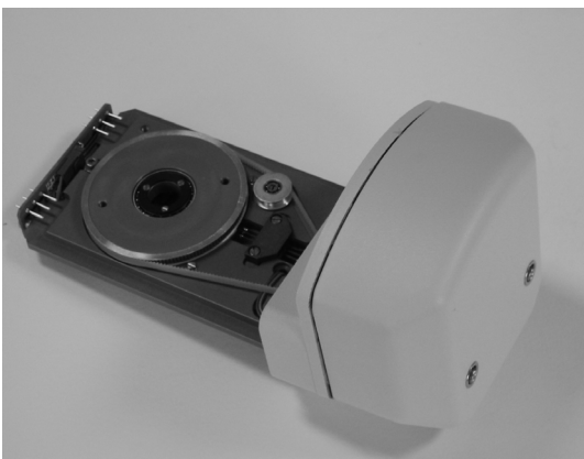
Figure 38: a) Automatic Knife Edge Aperture with Housing b) without Housing
