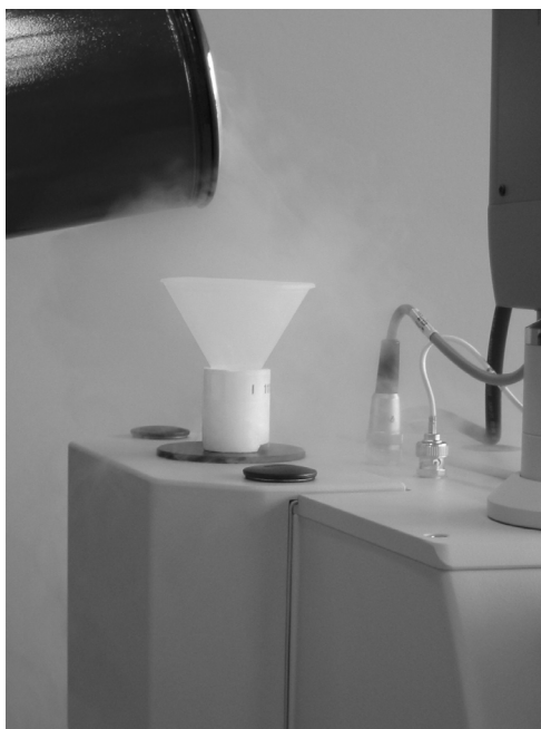
Figure 26: Filing the MCT Detector with Liquid Nitrogen
