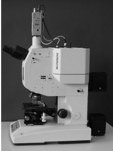
Figure 54: a) Accessory Port with Flange Cap b) HYPERION1000/2000 connected to Spectrometer
