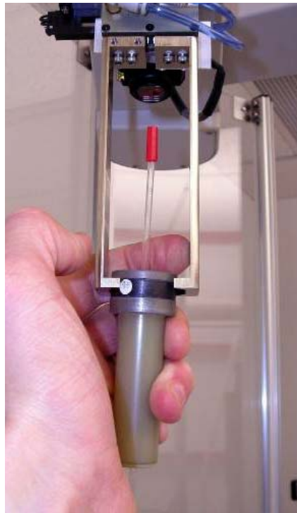
Figure 18 Manual removal of sample from robot gripper
