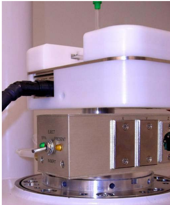
Figure 20 Manual Insert/Eject lever to be used in conjunction with Bypass button for manual insert/eject
