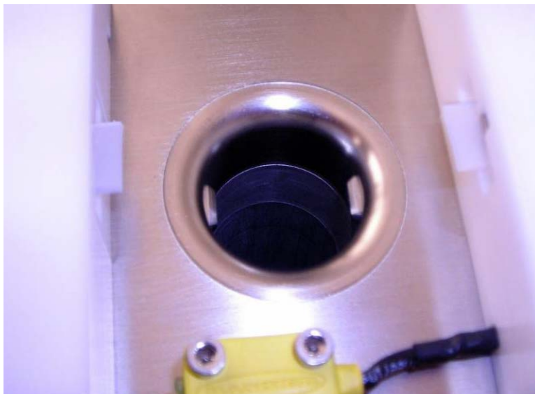
Figure 9 Upper Barrel module with sample catch mechanism engaged
