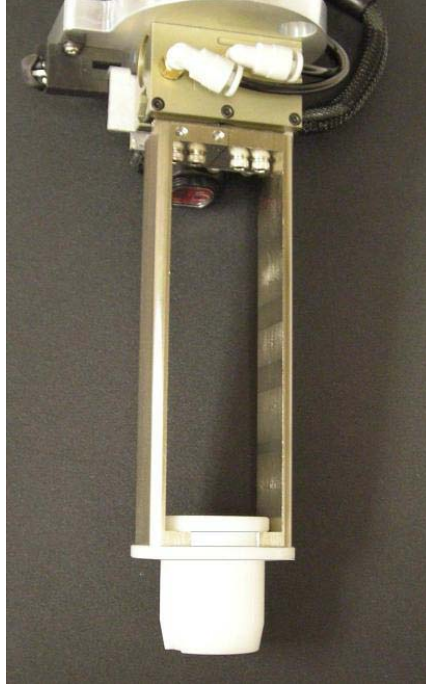
Figure 38 Insert upper barrel calibration tool
