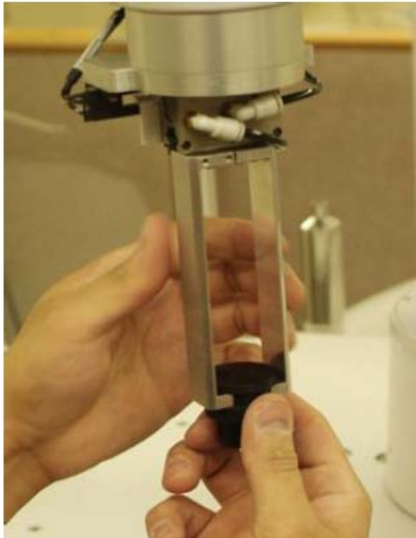
Figure 29 Tray teaching tool in gripper
