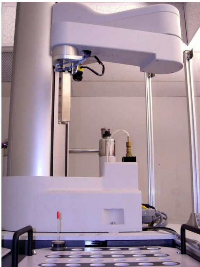
Figure 15 Left-handed orientation is incorrect, the system does not operate in this orientation
